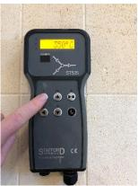
3 – Press the step key again, which will show the temperature the damper will close at. \*
