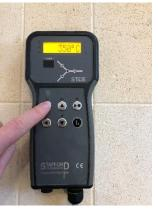
5 - Press the step key again, which will show the temperature the damper will open at. \*
