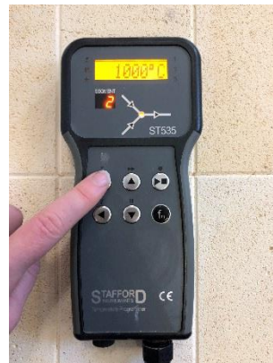
8 - Pressing the step key takes us to the target temperature in °C/hr.
