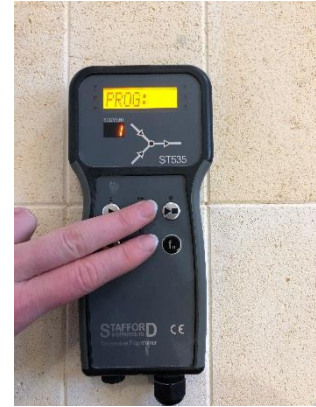
3 - Change the programme number by pressing either the up or down arrow.
