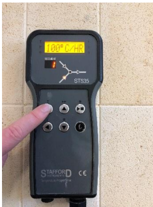
4 - Pressing the step key will take us to the heating ramp - how fast the kiln rises in °C/hr.
