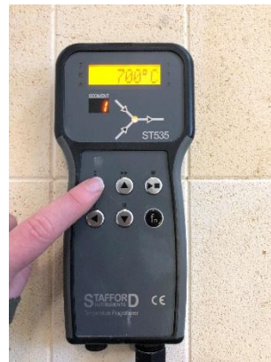
5 - Pressing the step key takes us to the target temperature in °C/hr.
