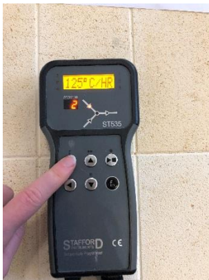
7 - Pressing the step key takes us to segment 2 - the second heating ramp in °C/hr.
