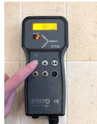
9 - Pressing the step key takes us to the soak or hold at temperature e.g. 00hs.20mins.
