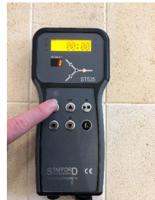
6 - Pressing the step key takes us to the soak or hold at temperature e.g. 00hrs.00mins.
