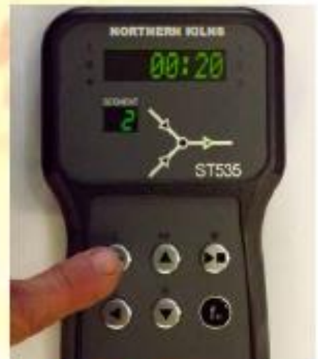
(9) Pressing the STEP key again will progress us to the soak at temperature or hold at temperature, in this case no hold or 20 minutes (00 hrs : 20mins)
