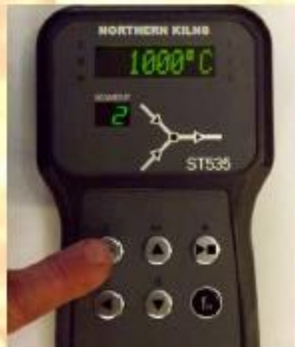
(8) Pressing the STEP key again will progress us to the target temperature, in this case 1000°C. To change the value press the up or down arrow.
