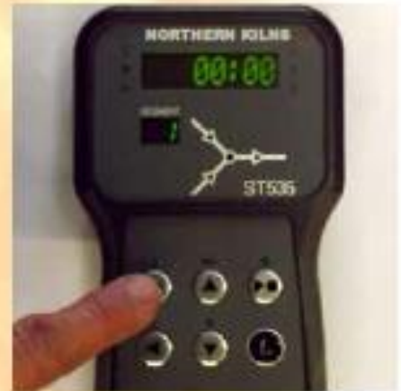
(6) Pressing the STEP key again will progress us to the soak at temperature or hold at temperature, in this case no hold or (00 hrs .00mins)
