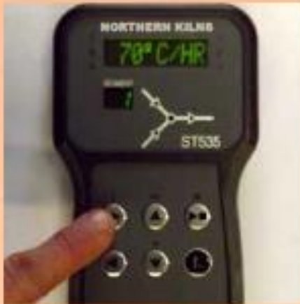
(4) Pressing the STEP key again will progress us to the heating ramp or how fast the temperature rises in degrees centigrade per hour (°C/hr). To change the value press the up or down arrow.
