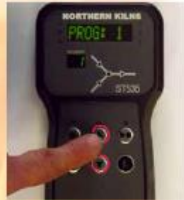
(3) Change programme number (32 in total) by pressing either up or down arrow key.
