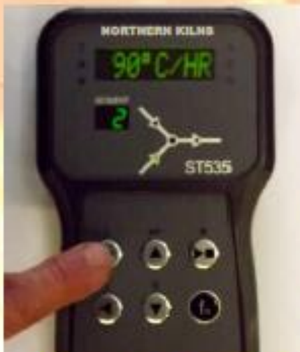
(7) Pressing the STEP key again will progress us to segment 2 or the second ramp, heating ramp or how fast the temperature rises in degrees centigrade per hour (°C/hr). To change the value press the up or down arrow.
