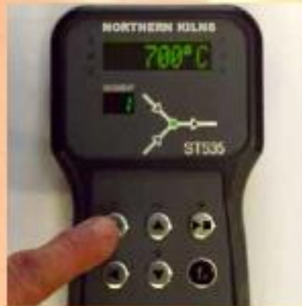
(5) Pressing the STEP key again will progress us to the target temperature, in this case 700°C. To change the value press the up or down arrow.
