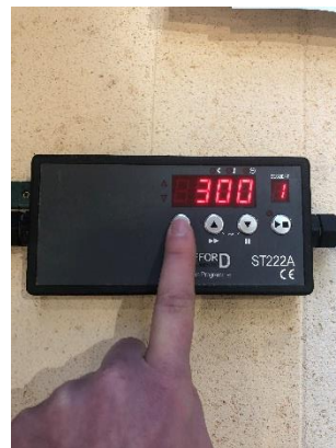
5 - Pressing the step key will take us to the heating ramp - how fast the kiln rises in °C/hr.
