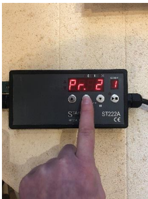
4 - By pressing the up arrow key, we have changed to programme number 2.
