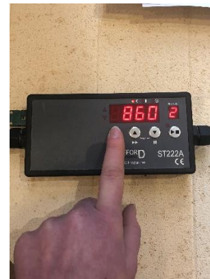
8 - Pressing the step key takes us to segment 2 - the second heating ramp in °C/hr.
