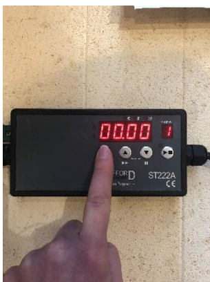
7 - Pressing the step key takes us to the soak or hold at temperature e.g. 00hrs.00mins.
