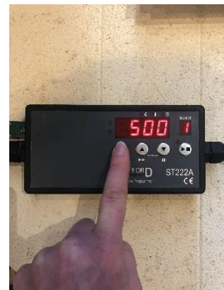
6 - Pressing the step key takes us to the target temperature in °C/hr.
