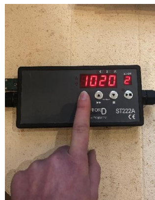
9 - Pressing the step key takes us to the target temperature in °C/hr.
